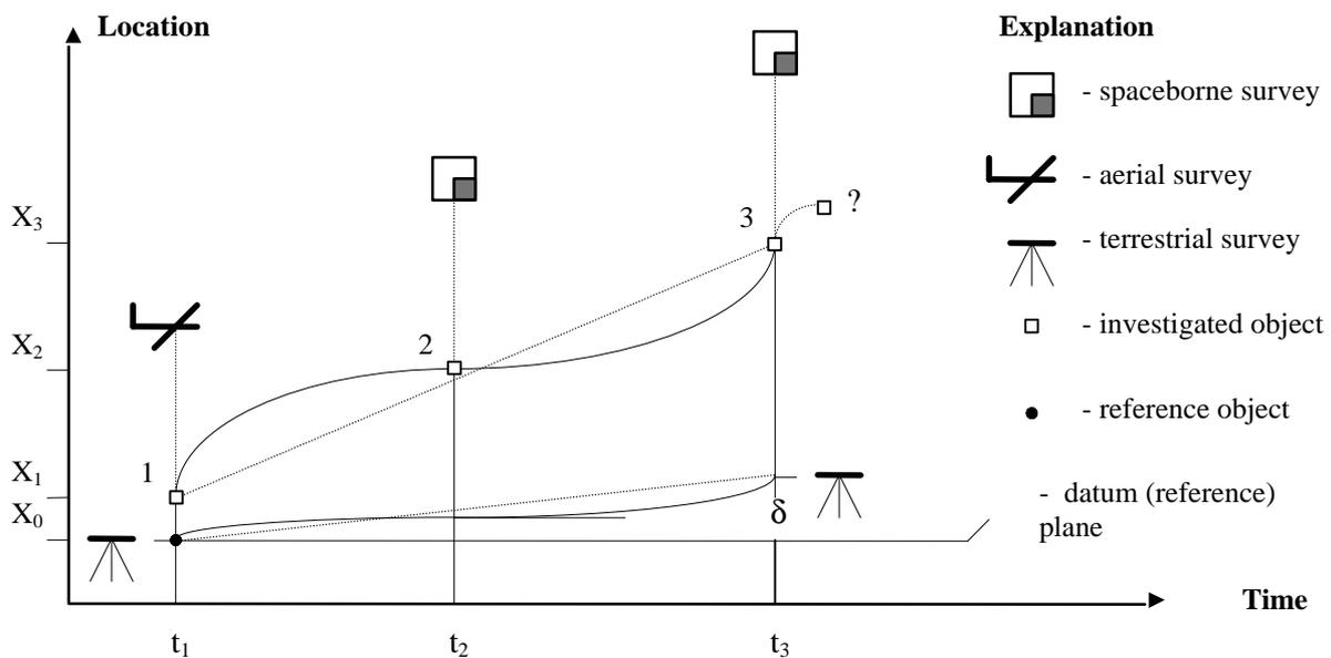
Figure 9. Concept of multistage surveys for coastal hydrographic monitoring
