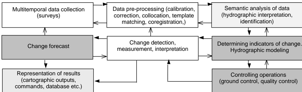
Figure 1. Principal flow chart of satellite monitoring
